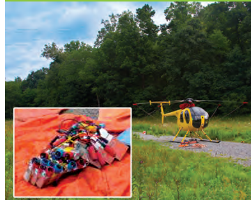
Hawk field stations, batteries and VectorSeis sensors can be placed in equipment bags and transported by helicopter to quickly reach receiver locations.
