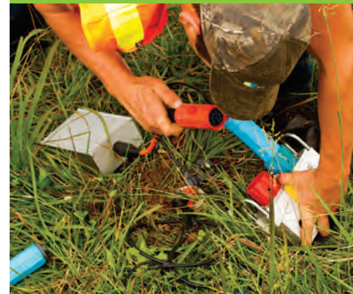
Crew member connecting the battery to a Hawk FSU during deployment at the receiver location.
